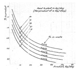
"From these curves it can be seen that the maximum attainable production of 1% material would be a trifle under 10 kilos per day, and this would involve a very large quantity of feed material, with a very high concentration of 25 left in the reject. Probably it would be unwise to try to lower the concentration of 25 in the rejected material below
