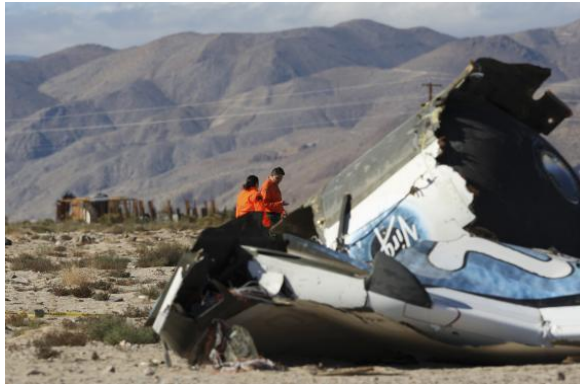
Fig. 2 - Crashed vehicle has a carbon composite fuselage. It is interesting that not one single wire or cable is visible in this photo. (Photo credit: Reuters)
